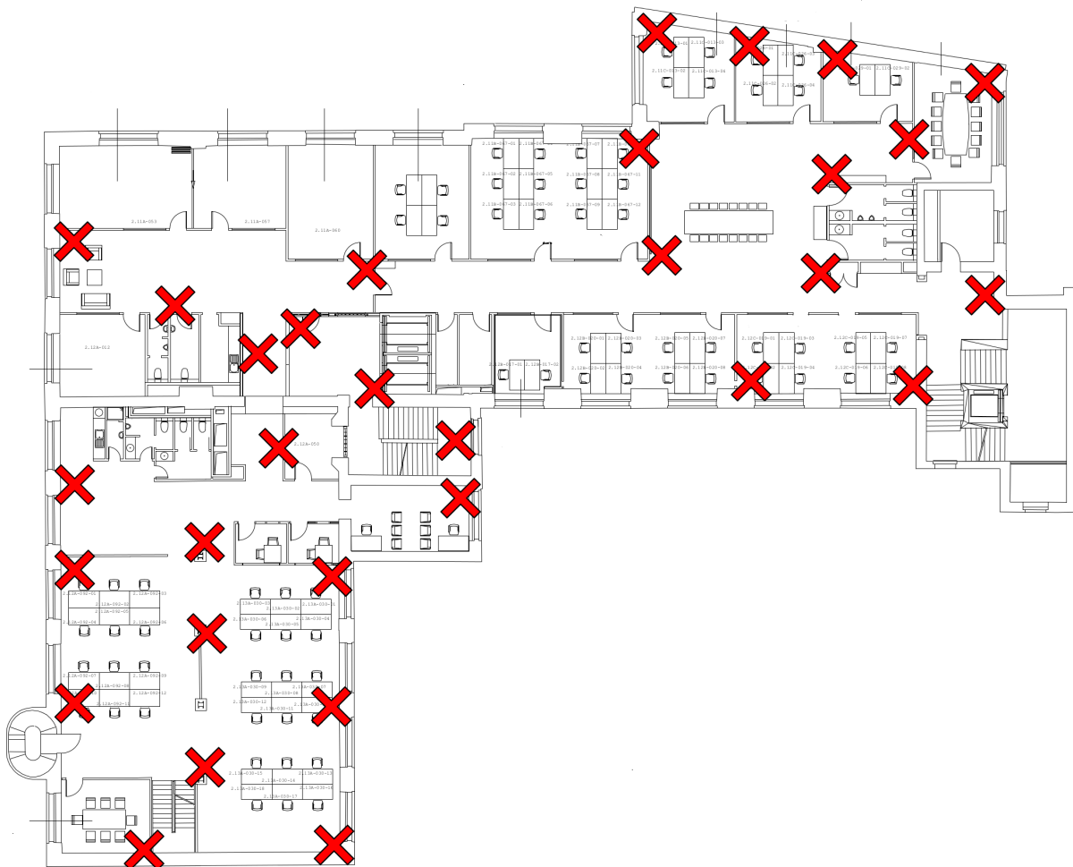
Figure 2: Exemplary Beacon Deployment
