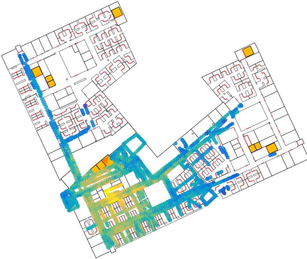
Figure 4: Radio data for one Wi-Fi Access Point collected with HERE Indoor Radio Mapper
