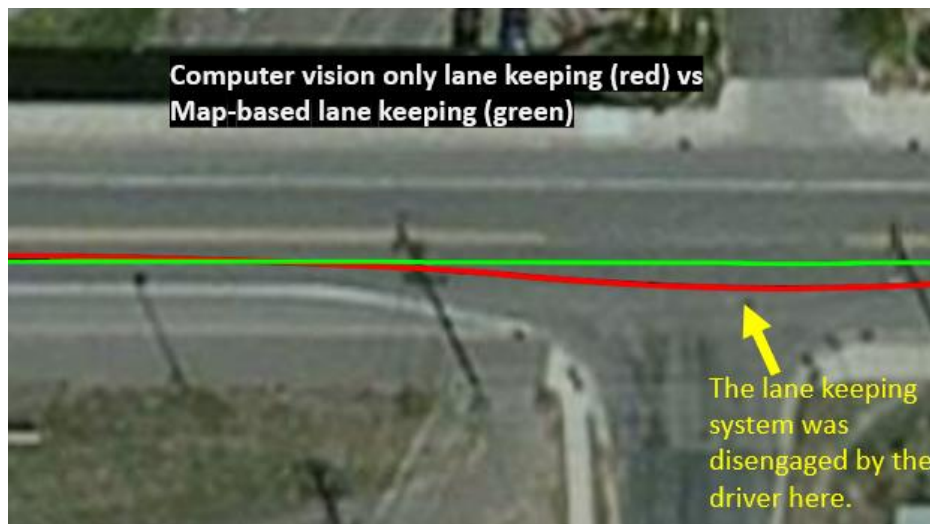
Figure 12: This image shows a comparison of the recorded paths the vehicle traveled with the computer vision only lane keeping system (red) and the map-based lane keeping system (green).
